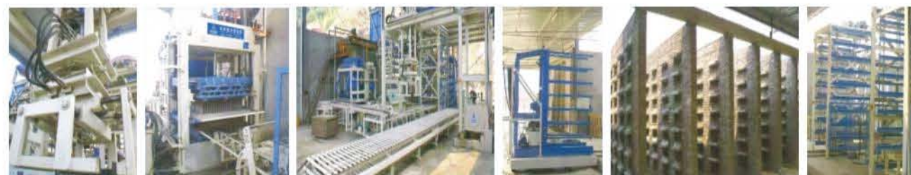
Curber system Forming system Working site Figer carts Curing room Elevator & lowerator
